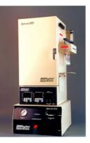
SFE is an alternative technique using supercritical carbon dioxide to extract additives from polymers. It reduces the use, exposure to, and disposal of hazardous solvents, while providing comparable extraction results in less time. This application describes the extraction of antioxidant from high density polyethylene using supercritical fluid.
