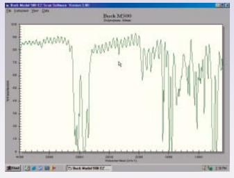
EZ-Scan Software provides complete control of Instrument Parameters and basic Data Processing; where Spectra can be overlaid for comparison, data can be exported as X/Y ASCII files, the active cursor provides precise Wavelength/ABS values, etc.
