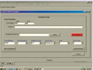
Operator-control of the Scan Range, Wavelength setting, Collection Mode, Timing and Signal Processing are all available through our proprietary instrument interface
